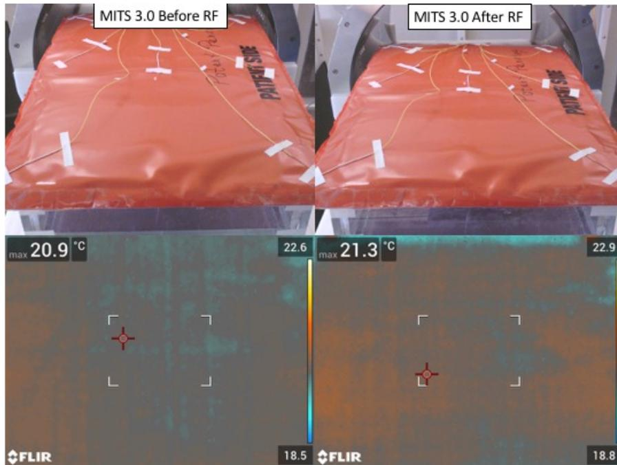
**Figure 2: Image showing heating before (left) and after (right) RF exposure at 128 MHz (3.0 T).** The thermal camera images (lower row) show no evidence of any significant localized heating not captured by the fiber-optic sensors.
