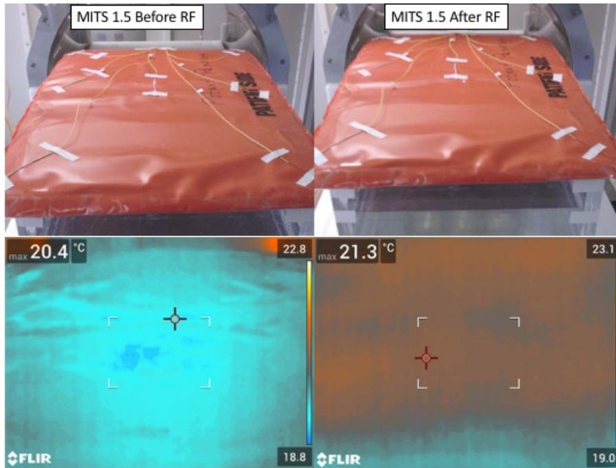
**Figure 1: Image showing heating before (left) and after (right) RF exposure at 64 MHz (1.5 T).** The thermal camera images (lower row) show no evidence of any significant localized heating not captured by the fiber-optic sensors.
